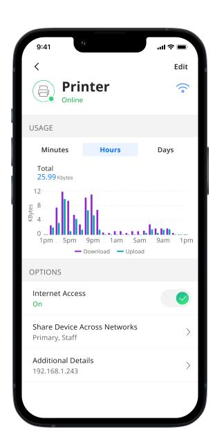
The Device details screen shows the device name at the top of the screen followed by a chart that indicates the amount of data that was used by the device over a period of time.
