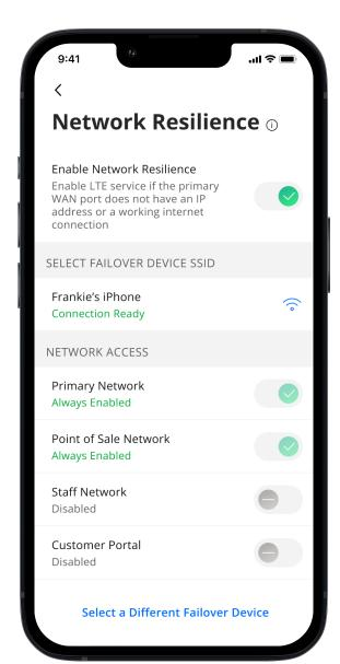
From the My Network screen, tap **Network Resilience** to select a mobile device to provide secondary cellular/LTE service for your most critical networks during internet outages.
